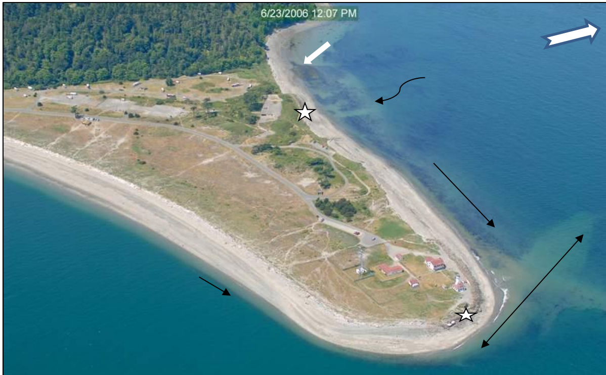
LOCATION A, development of Point Wilson. The relative strength of the longshore drift currents is indicated by the length of the black arrows; double-ended arrow is tidal current. Riprap (stars) at the Coast Guard facilities and Battery Kinzie fails to stop gradual southward movement of the spit. Simple white arrow indicates Location B, the “drowned forest”. Mystery features are at the curved arrow. (2006 Washington Dept. of Ecology aerial oblique photo)
